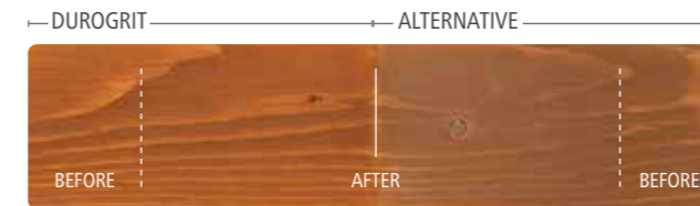
The colour Foxy Brown on pine tested for UV protection after 5 years against an alternative product using a two-layer system.
