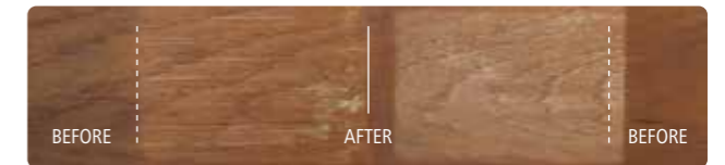
The colour Grassland Beige on teak tested for UV protection after 5 years against an alternative product using a two-layer system.
