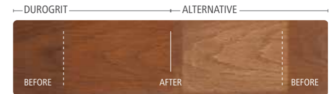
The colour Foxy Brown on teak tested for UV protection after 5 years against an alternative product using a two-layer system.
