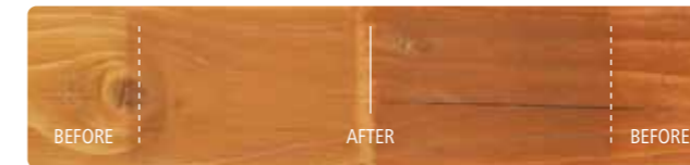
The colour Grassland Beige on pine tested for UV protection after 5 years against an alternative product using a two-layer system.
